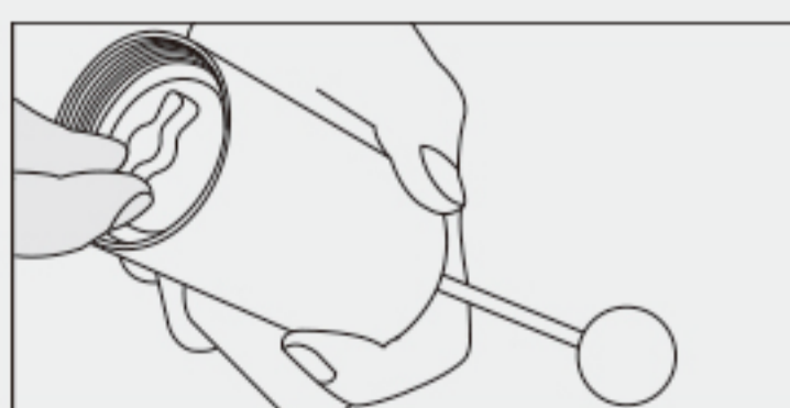
Rotate the adjusting plate counterclockwise to grind coarse powder; clockwise to fine powder
